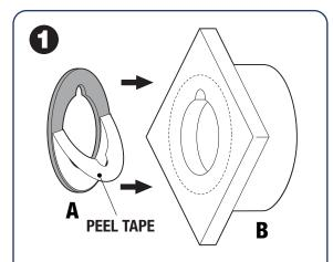
Mark where hole is to be drilled. Remove paper on one side of the mounting tape **(A)** and stick to the bottom of the Drill Guide **(B)**, aligning holes.
