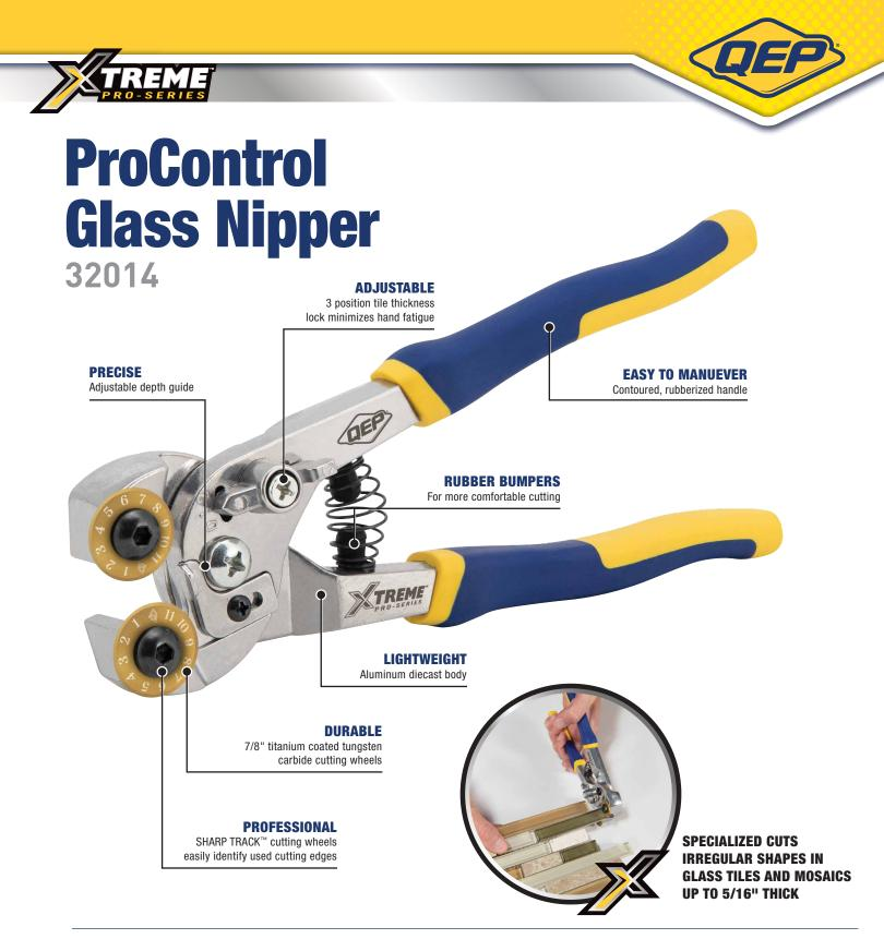
The QEP® Xtreme<sup>™</sup> Series 8.25" Glass Tile Nipper is professionally engineered to shape irregular glass and tile mosaics up to 5/16" thick. Easily snip away at pieces with tough, titanium coated tungsten carbide cutting wheels. Sharp Track<sup>™</sup> design identifies used cutting edges to maintain a hard cutting edge. 3 Pro Control settings make this nipper easily adjustable.
