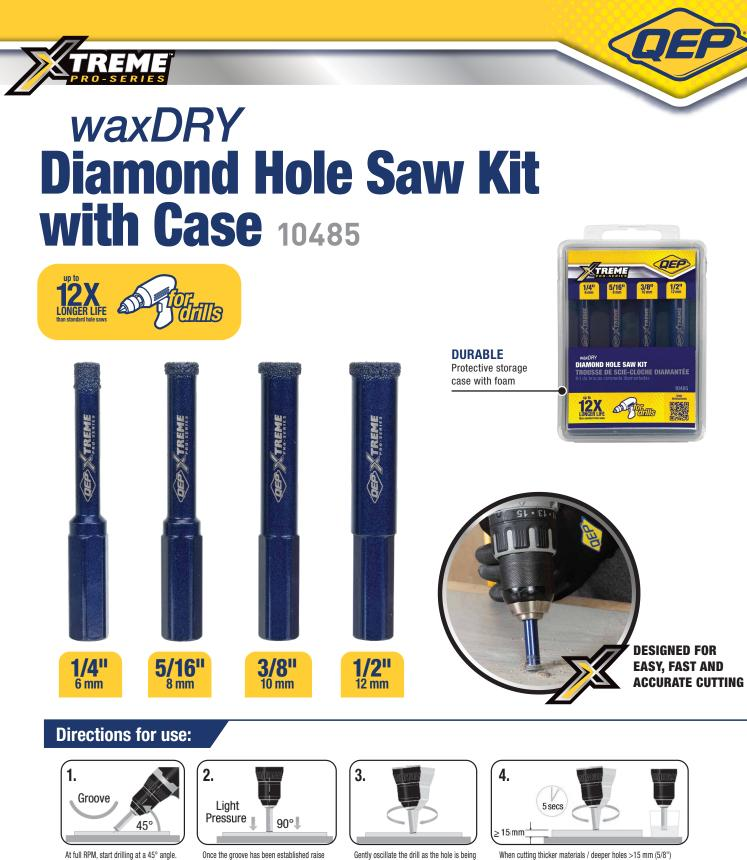
When cutting thicker materials / deeper holes >15 mm (5/8") additional cooling is required. Dip the hole saw into water every 5 seconds during cutting.
