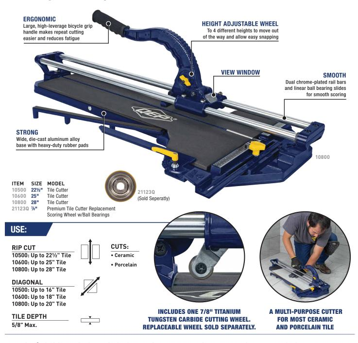
The QEP® Big Clinker Tile Cutter Series is a multi-purpose cutter for most ceramic and porcelain tile. These cutters have Ishii engineering with a wide cast aluminum alloy base with heavy rubber pads for cutting stability, dual chrome-plated rail bars and linear ball bearing slides for smooth scoring. The base includes side arm extensions to support large format tiles.
