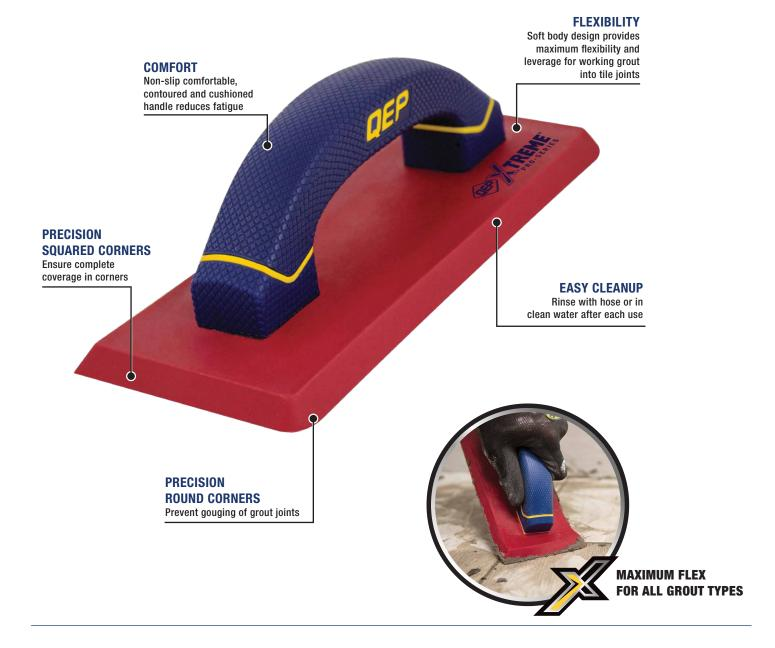
The QEP® Stone Grout Float can be used with all types of grout and tile, making it a versatile tool for your installation projects. This grout float will not mar or scratch tile. The beveled sides hold edge longer while the square sides ensure complete coverage in corners. The non-slip comfortable handle works well in either the left or right hand. 10" x  $3\frac{1}{2}$ ".
