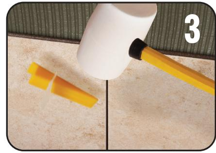
Once mortar has set, simply tap the clips with a non-marring rubber mallet to snap off at the specially designated break-points. Save wedges for future use.
