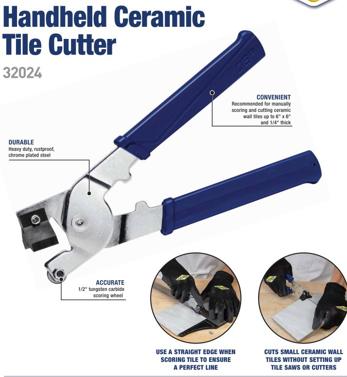
The QEP $^{\circ}$  Handheld Ceramic Tile Cutter is the perfect tool for manually cutting small ceramic wall tiles up to 6" x 6" and 1/4" thick. Quickly score and snap small tiles without using large tile cutters or saws. This tool includes one 1/2" tungsten carbide scoring wheel for durable and accurate tile scoring. To guarantee a perfect cut, run the scoring wheel up against a straight edge.
