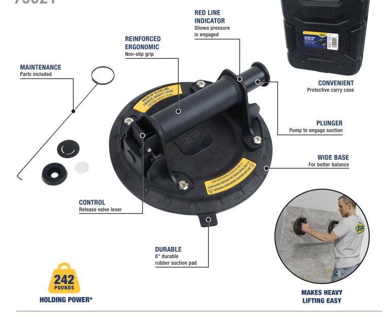
The QEP® 8" Vacuum Pump with Suction Cup makes heavy lifting easy. This hand held portable suction cup has a holding power of 242 lbs. It can be used to lift large tiles, stone, glass and all types of non-porous building material. To use, pump plunger until red line disappears and suction is engaged. During use, red line should not be not visible. Release valve is located on opposite end of plunger. Store with protector cover (included) in durable carrying case.
