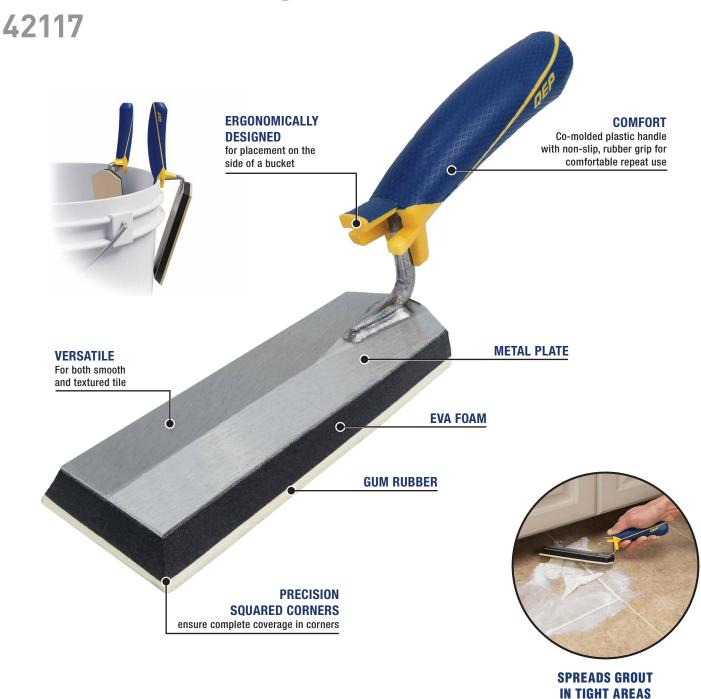
This installer grade QEP $^{\circ}$  6" x 2" Comfort Grip Margin Float is used for tile grouting in hard-to-reach areas, including back splash and under counters. It has a comfortable non-slip handle and a steel backing plate that resists bending. The padding is made of gum rubber, which is ideal for easily pushing grout into grout joints, due to its strength and flexibility.
