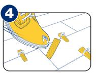
Once the mortar sets, break-off in direction of grout line within 24 hours
