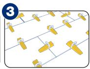
Secure wedge into clips to level, align space and hold the tiles
